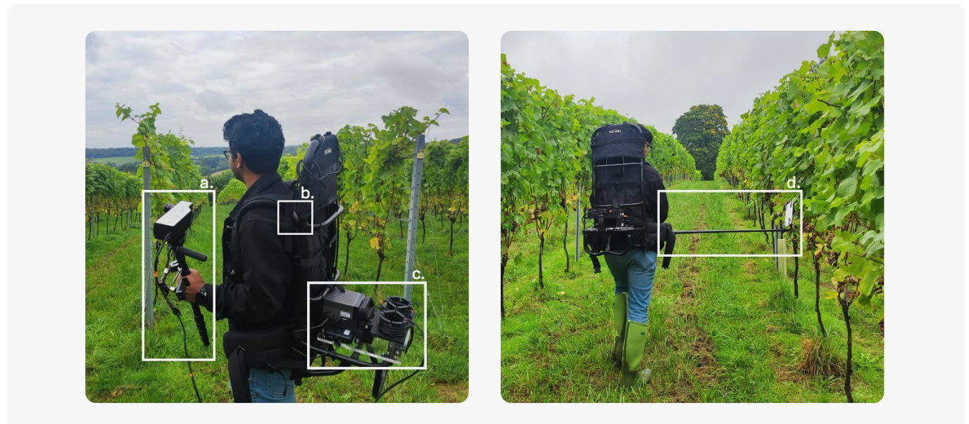
Annotated images showing: a. Living Optics camera on Monopod b. GPS BU-35 Backpack c. Living Optics Development Kit d. Telescopic pole with white reference. The set-up weighs around 8 kg.
